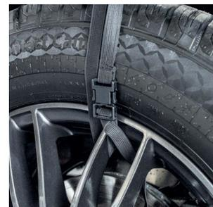
In addition, there are loops on the windshield insulation for another guy on the rims. Guide the rubber strap through the loop and an opening of the rim and close the click lock. Again, you can readjust the strap and tighten it as tight as necessary. Now do the same on the other side of the vehicle.
